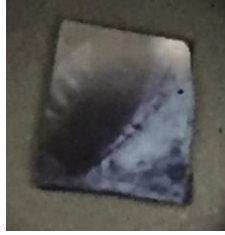
Figure E.1: Cu-BTC/Al 2 O 3 /p-Si. The thin film shown here is 40 cycles thick.
